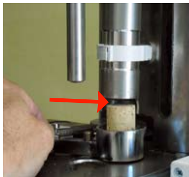
Fig. 3. Adjust Cork Descent Tube if Cork Length is NOT 1-3/4"
