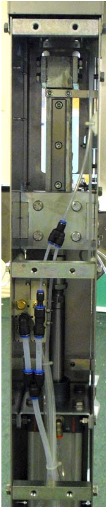
Fig. 6. Back of corker. Lubricate rail annually.
